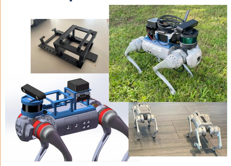
Background: For a research lab, additional computers and sensors needed to be onboard quadruped robots to support experiments. A compact "backpack" to mount the components was required.
